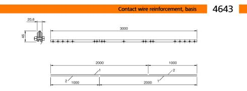
**Note:** Tightening torque: Bolt M 10 MA = 25 Nm
